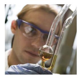
Fluid monitoring and LubeWatch® oil analysis are excellent methods to help track the health of your lubricating system, but while they can detect varnish precursors in your oil stream, they can't usually detect varnish that has already formed.
